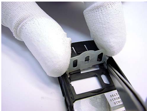
Press with tweezers one side from the SIM Card Holder and remove it.
