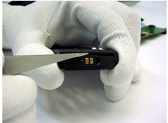
Turn round the B-Cover. If the System Connector is jammed, press with tweezers between cover and connector.
