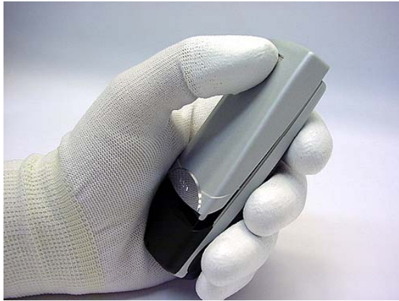
Press the lock-button and push the Battery Cover in direction to the System Connector.
