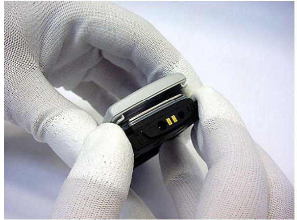
Pull back the A-Cover from the bottom side on and remove it.
