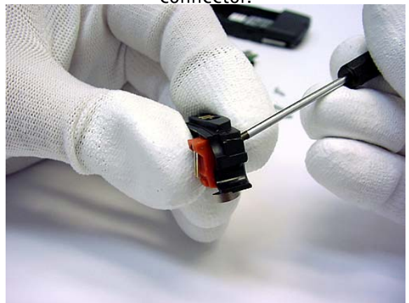
Press the Vibra Motor with a screwdriver out of the System Connector.
